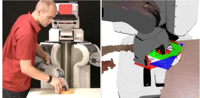
Fig. 1. User demonstrates an appropriate grasp candidate to the PR2 robot (left). A visualization of the corresponding template extracted from the perceived point cloud along with the corresponding gripper pose is shown on the right.
