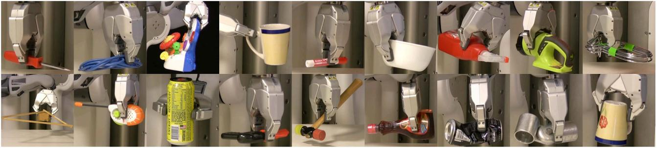
Fig. 7. Subset of the achieved grasps on the test set on the PR2.
