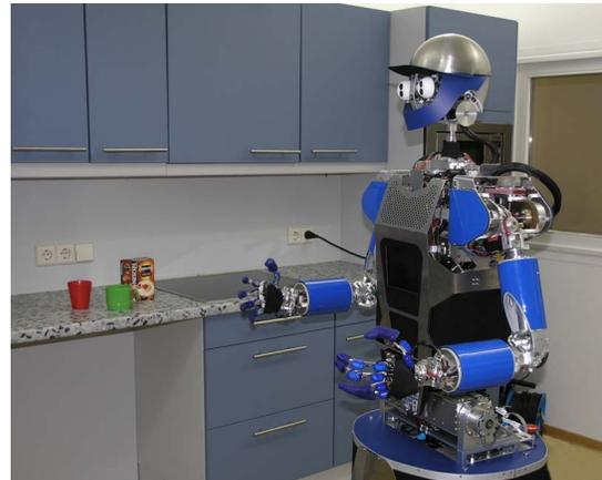
Fig. 1. The humanoid robot ARMAR-III.
